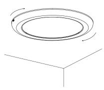
Aim the groove at the installation bracket, rotate the lamp clockwise until it is firmly fixed, turn on.
