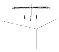
Knock-in the plastic anchor into ceiling, fix bracket with screw.
