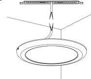
Connect wires with L,N, and do insulation treatment.
