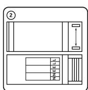
Insert screwdriver to release cord grip to gain access to tool-less terminals.
